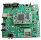
The 516-CN Mounted on Development Kit Carrier Board
