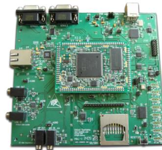
The 516-CN Mounted on Development Kit Carrier Board
